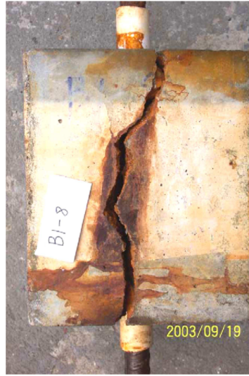
Fig. 2.29 Splitting failure of corroded specimens (Fang et al. 2006)
