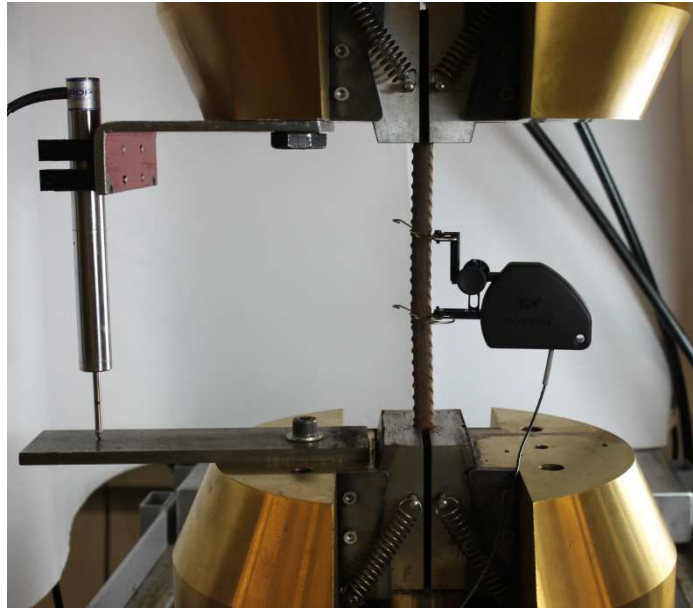
Fig. 3.6 Buckling test setup
